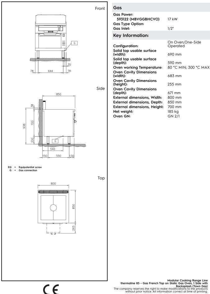
Modular Cooking Range Line thermaline 85 - Gas French Top on Static Gas Oven, 1 Side with Backsplash (Town Gas) The company reserves the right to make modifications to the products without prior notice. All information correct at time of printing.
